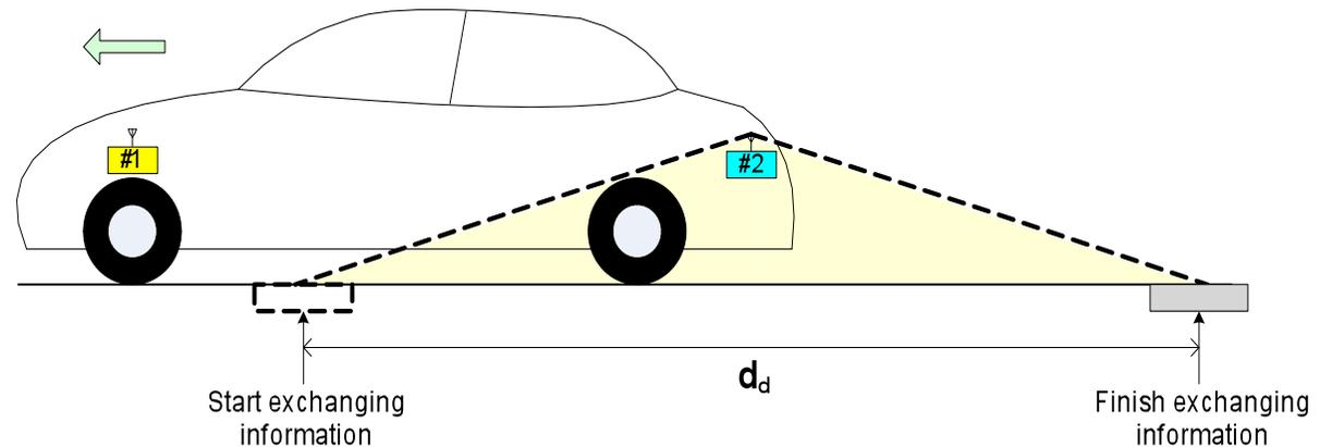
$t_{ad}$  denotes the maximum time available for the vehicle and the belt to establish data exchange successfully at a given speed
