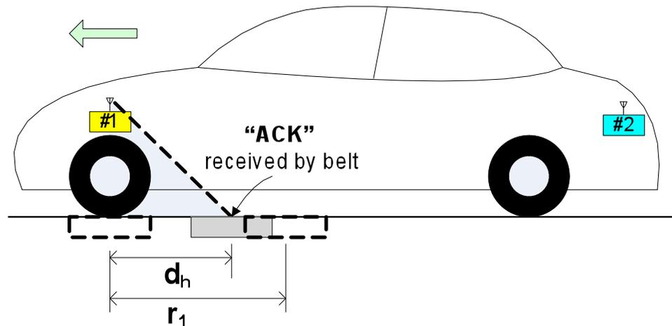
$t_{ah}$  denotes the maximum time available for the vehicle and the belt to establish handshaking successfully at a given speed
