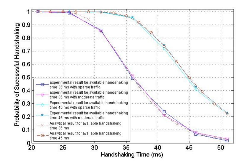
Connection Setup and Handshaking 3)  $t_h = 36$  ms,  $\mu$  is varied,  $T_{ah} = 36$ , 45 ms
