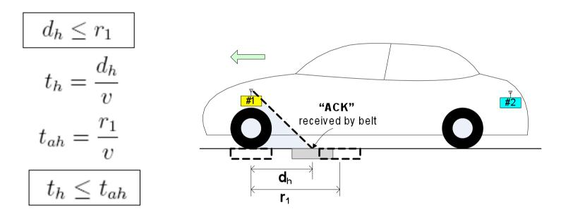
$t_{ah}$  denotes the maximum time available for the vehicle and the belt to establish handshaking successfully at a given speed
