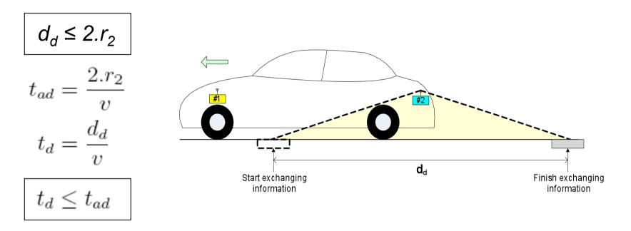
$t_{ad}$  denotes the maximum time available for the vehicle and the belt to establish data exchange successfully at a given speed
